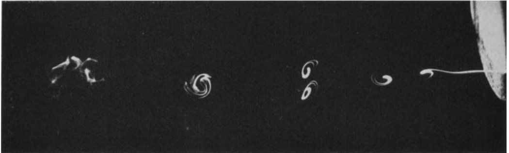
FIGURE 1. Instantaneous photograph of the rolling-up process of vortices, of slipping and coalescing of vortices, and of vortex disintegration. The smoke was introduced into the separated layer of an axisymmetric jet. D = 7.5 cm, U_0 = 3 m/sec, f = 95 Hz.
